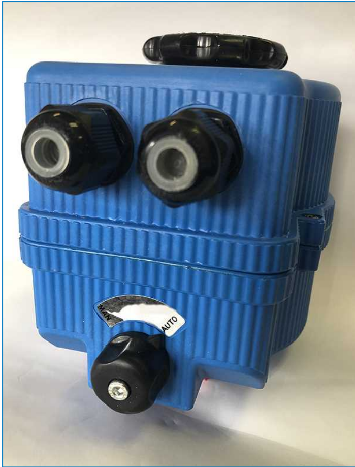
Purge valve actuator position "AUTO"
