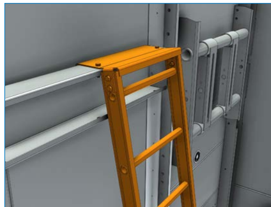
Lift the ladder into place and drop the pre-welded bolts into the mounting holes in the upper support channel. No further fastening is required.
