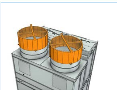
Lift single discharge attenuator onto the pre-installed fan cowl.
