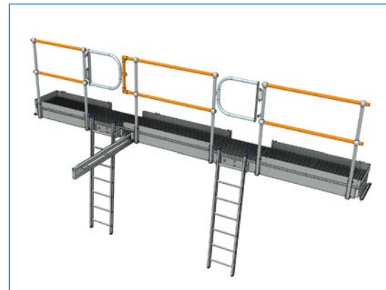
Slide in the horizontal tubes into the vertical posts, secure with hardware installed in vertical post
