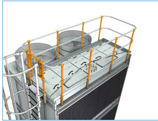
Install all vertical posts.
